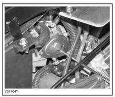
Insert the needle of lubricant can in the end of throttle cable adjuster.
