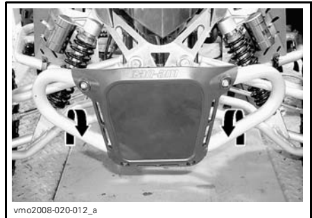
DS 90 X — FRONT ATTACHMENT LOCATION
