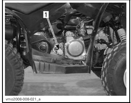
TYPICAL — RH SIDE OF ENGINE 1. Dipstick
