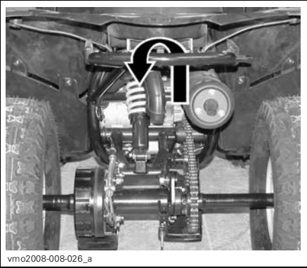
ALL MODELS — REAR ATTACHMENT LOCATION
