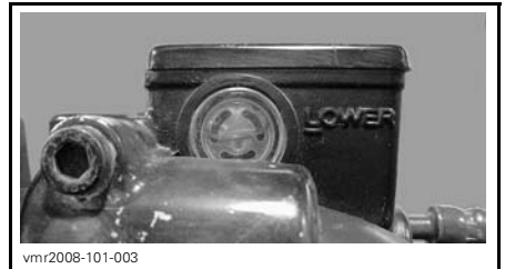
LH REAR BRAKE FLUID RESERVOIR
