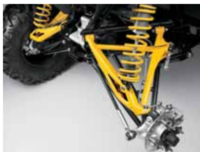
Torsional Trailing A-arms (TTA) independent rear suspension
