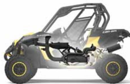
Rotax 1000R V-Twin engine with high-flow dynamics
