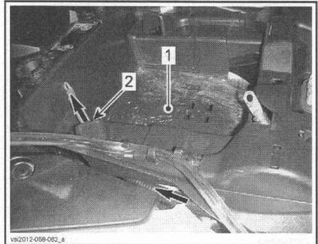
BATTERY REMOVED FOR CLARITY 1. Battery tray 2. Battery tray positive cable opening
